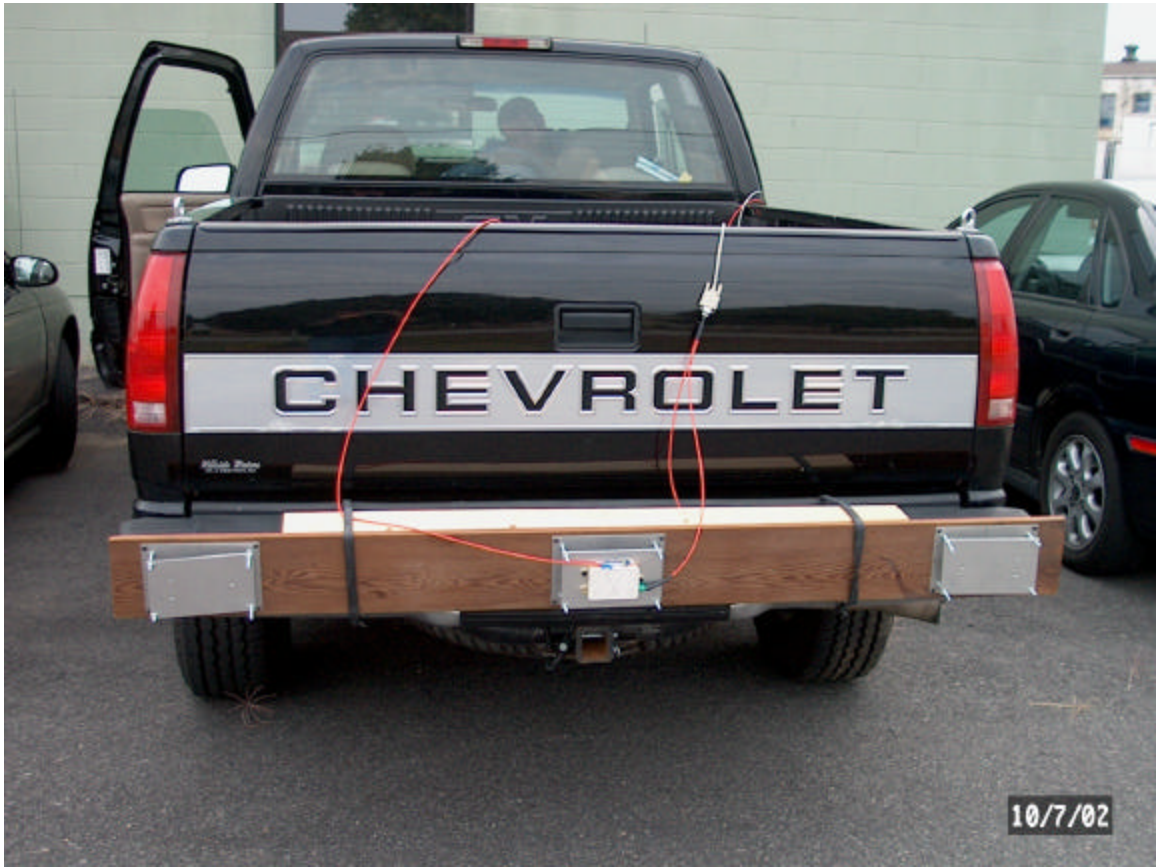
Figure 2 Photo of HRR sensor attached to mock automobile bumper for vehicular collision-avoidance testing.
